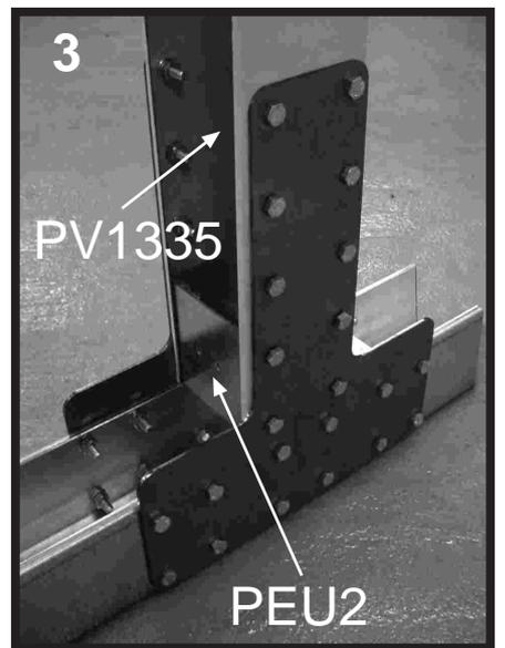
**EN** **COLUMNS (C) ASSEMBLING: 1°** - Assemble the two uprights using the following parts: 1 PV1335 + 1 PG + 2 PEAO + 2 PEU2 and TV screws.
