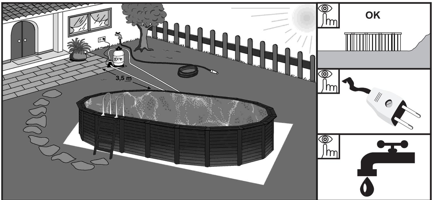
**EN** **Installation place:** Our pools are designed to be erected above ground and for an outdoor family use. The ground has to be firm, flat and perfectly horizontal. **Remember:** 1000 lts of water = 1 m<sup>3</sup> = 1000 Kgs.
