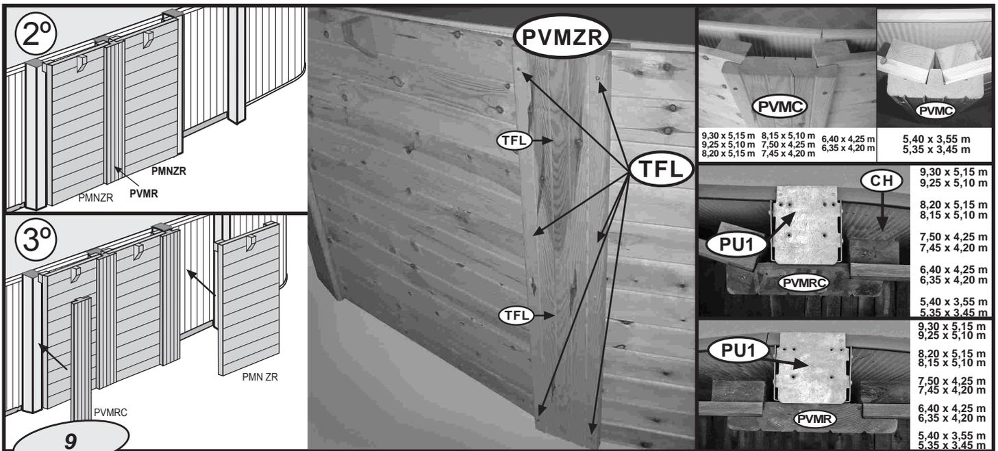
**EN** Once the panels have been attached to the curved sections, proceed with the straight sections.
