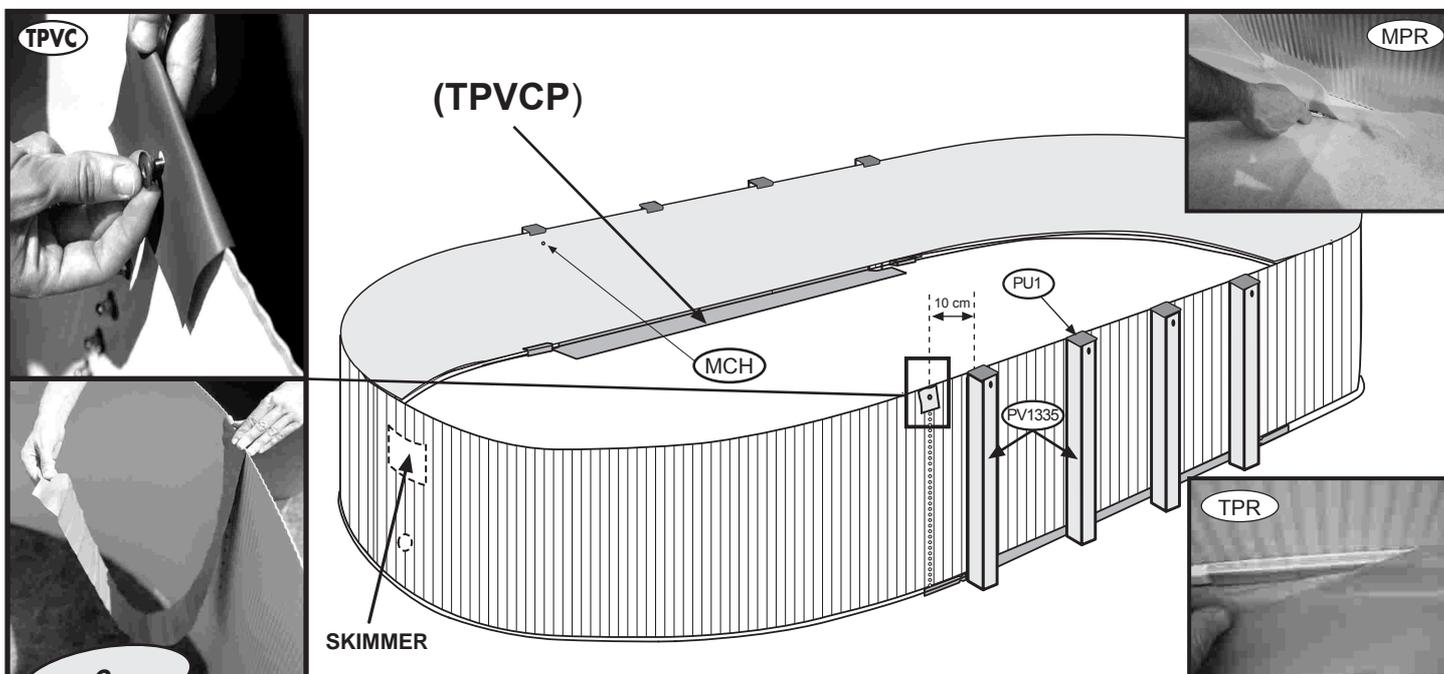
**EN** **PVC PROTECTIVE STRIPS (INSIDE OF POOL):** The pool is supplied with 2 wide PVC strips and 1 narrow one. The narrow strip must be attached to the top nut at the join of the wall plating and hung down inside to cover the screw heads. The 2 wider strips must be taped on to cover the metal brackets inside the straight part of the pool. All these strips are intended to protect the pool liner.
