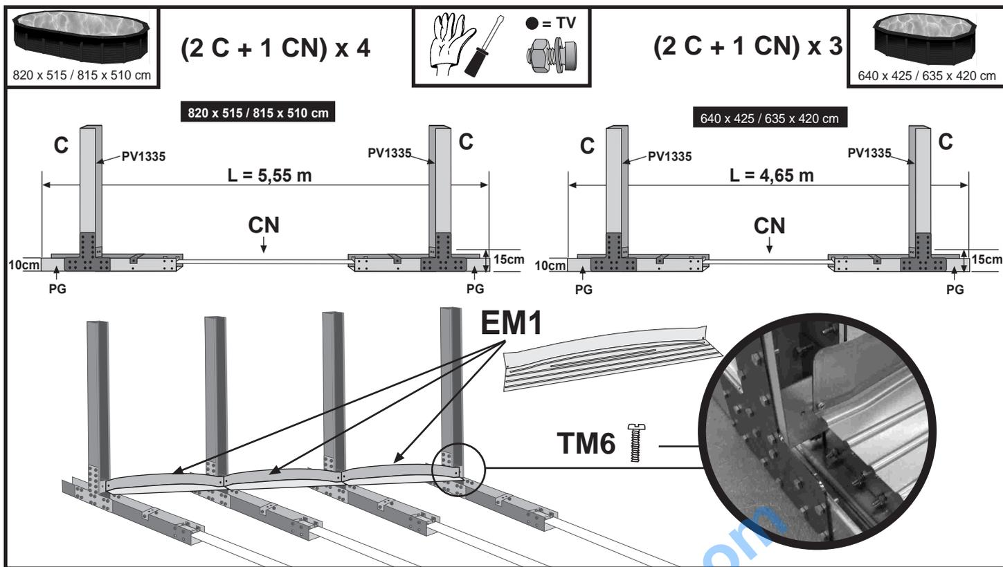
**EN** PROVISIONAL ASSEMBLY OF THE BRACKETS (EM1) ON THE UPRIGHTS (C).
