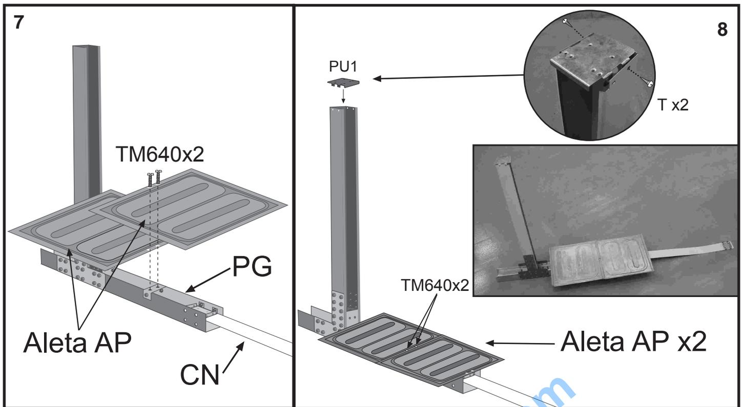
**EN** 7 – Place a **plate AP** so that its two holes coincide with the two holes in the part PEU. Then place the other part **AP** and fasten it using 2 **TM640** screws. (Before fitting the plates **AP** it is best to introduce the assembled beams in the ditch already prepared).
