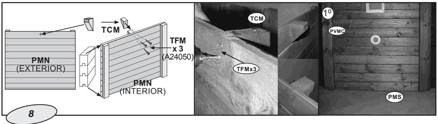
**EN** **WOODEN PANELLING – PLEASE NOTE:** When assembly does not begin immediately, it is important to restack the components horizontally on the pallet and cover them fully to ensure that sunlight and water do not penetrate. **Assembly of wooden panelling:** It is recommended that 2 adults wearing gloves perform the assembly.
